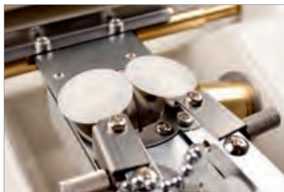
Both lens guides are fitted with plastic rollers each of which can be finely adjusted to ensure the precise position above the grooving wheel
